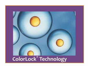
During drying of conventional paint the particles of colorants (yellow) adhere loosely to the resin molecules (blue).
