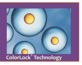
During drying of conventional paint the particles of colorants (yellow) adhere loosely to the resin molecules (blue).
